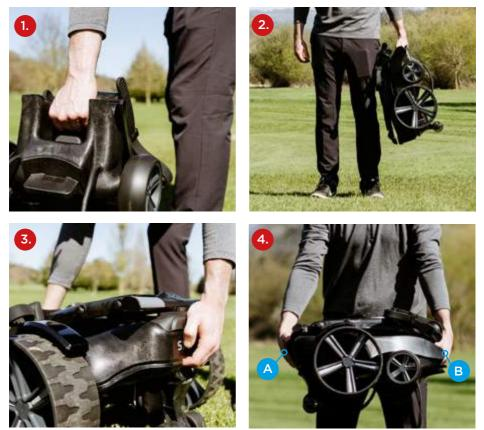
**Never** pick up the STEWART REMOTE by any points other than those described, doing so may cause damage. **DO NOT** lift by wheel arches.
